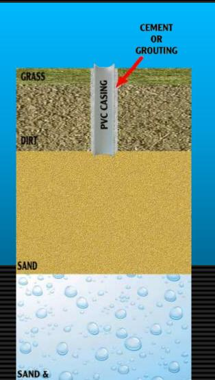
In around casing once in place with cement, grout or dirt, so casing is more secure.
