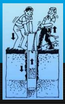
Insert casing into the hole and push in to depth drilled (follows bailing tool)
