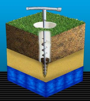
Once past thew soil the sand spear can be pushed into the ground by using a hammering effect
