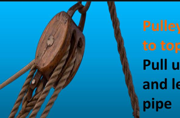
Pulley Block- Connect to top of tripod Pull up the weight and let it drop on the pipe
