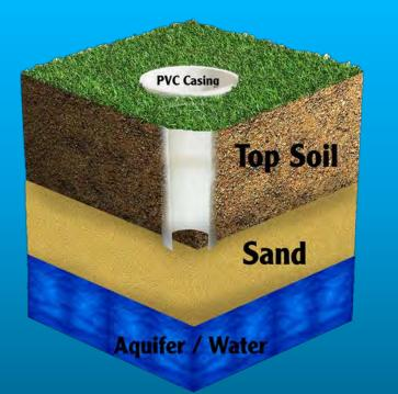
Insert protective casing to sand and water level as described above
