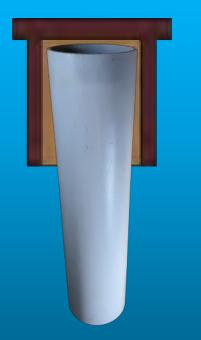
Safety Top cap This allows hammering effect to be put evenly on the riser, to stop cracking
