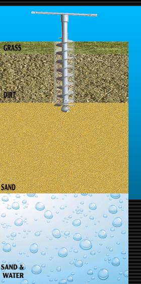
Auger Hole to the Sand & Water Aquifer
