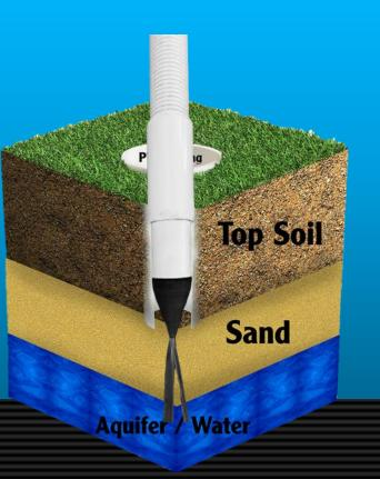
Pushing the casing by hand should be good enough to penetrate deeper into the sand
