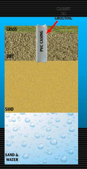
Fill in around casing once in place with dirt or cement in place so casing is more secured.
